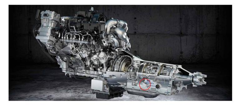
A new factory Ford F250 clip for the transmission shift linkage will be provided with this kit (This clip was removed at the end of **Step 3**. These clips are fragile when prying off, so if your factory clip broke that is okay).
